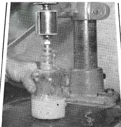
Taper reaming a 500 cc bottle to size B24. A badly choked bottle will be completed in 5-10 seconds
