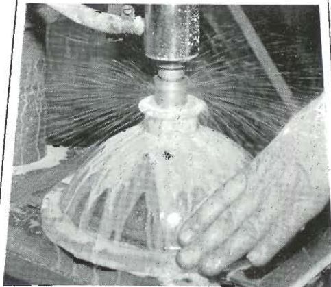
Taper reaming a borosilicate glass desiccator lid, size B34, at the works of Jencons (Scientific) Ltd., Hemel Hempstead. This operation is completed in only a few seconds. Tools can be supplied to both drill and ream out the hole in one operation
