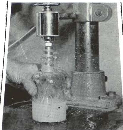
Taper reaming a 500 cc bottle to size B24. A badly chocked bottle will be completed in 5-10 seconds
