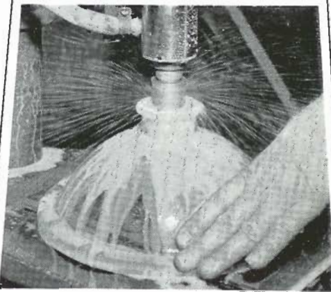
Taper reaming a borosilicate glass desiccator lid, size B34, at the works of Jencons (Scientific) Ltd., Hemel Hempstead. This operation is completed in only a few seconds. Tools can be supplied to both drill and ream out the hole in one operation
