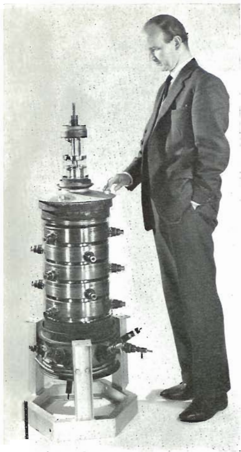
Figure 9 Complete 'five grid' mercury pool rectifier
